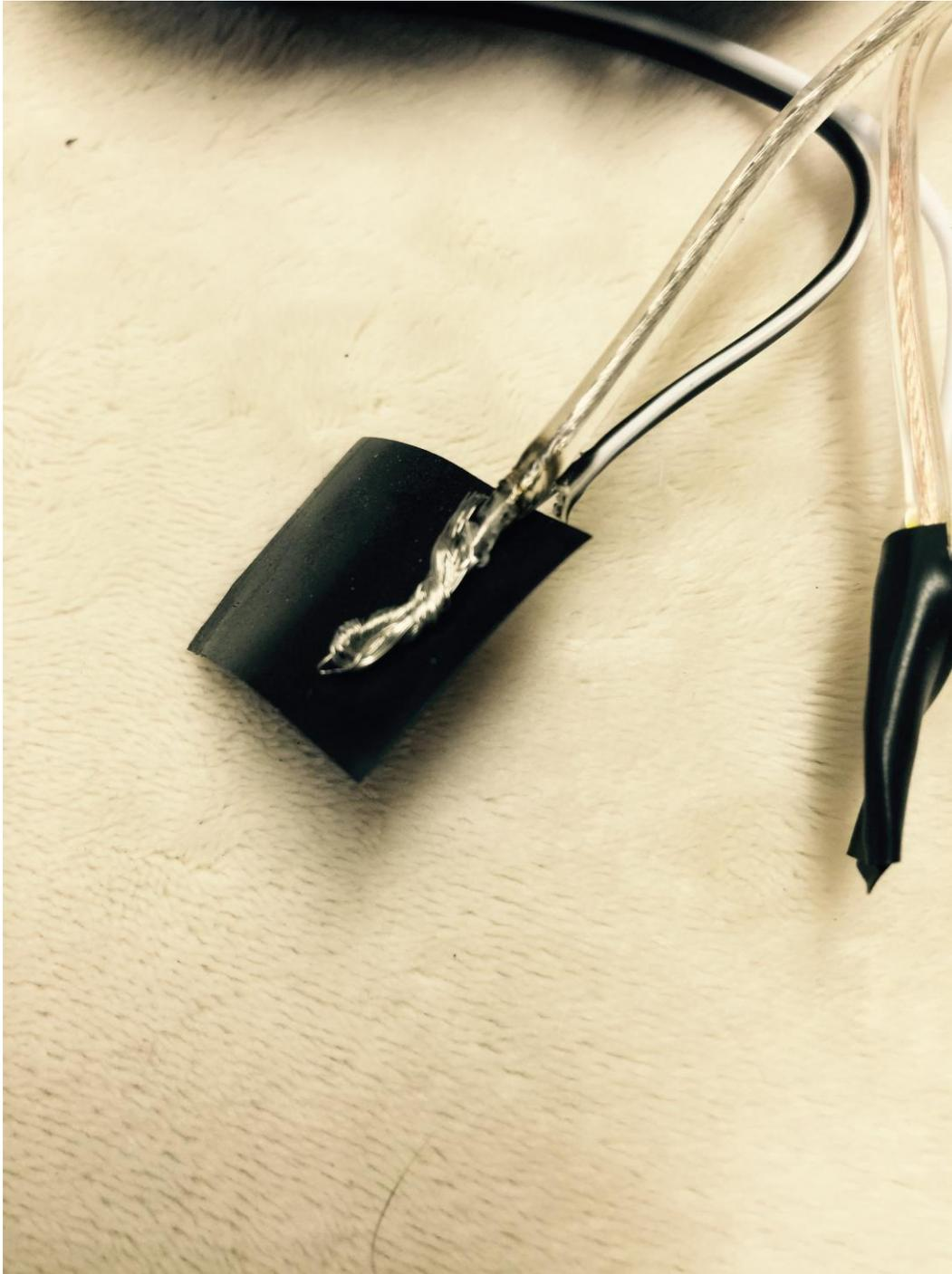
**Step three** is to tape the two wires taped referred to in step two above together insuring it will not allow any exposed wire to touch each other.
