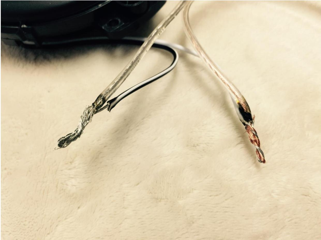
**Step Two** is using the electrical tape to cover the ½ half twisted wires where they have been joined to the puck. Be sure all of the exposed wire is covered by the tape.
