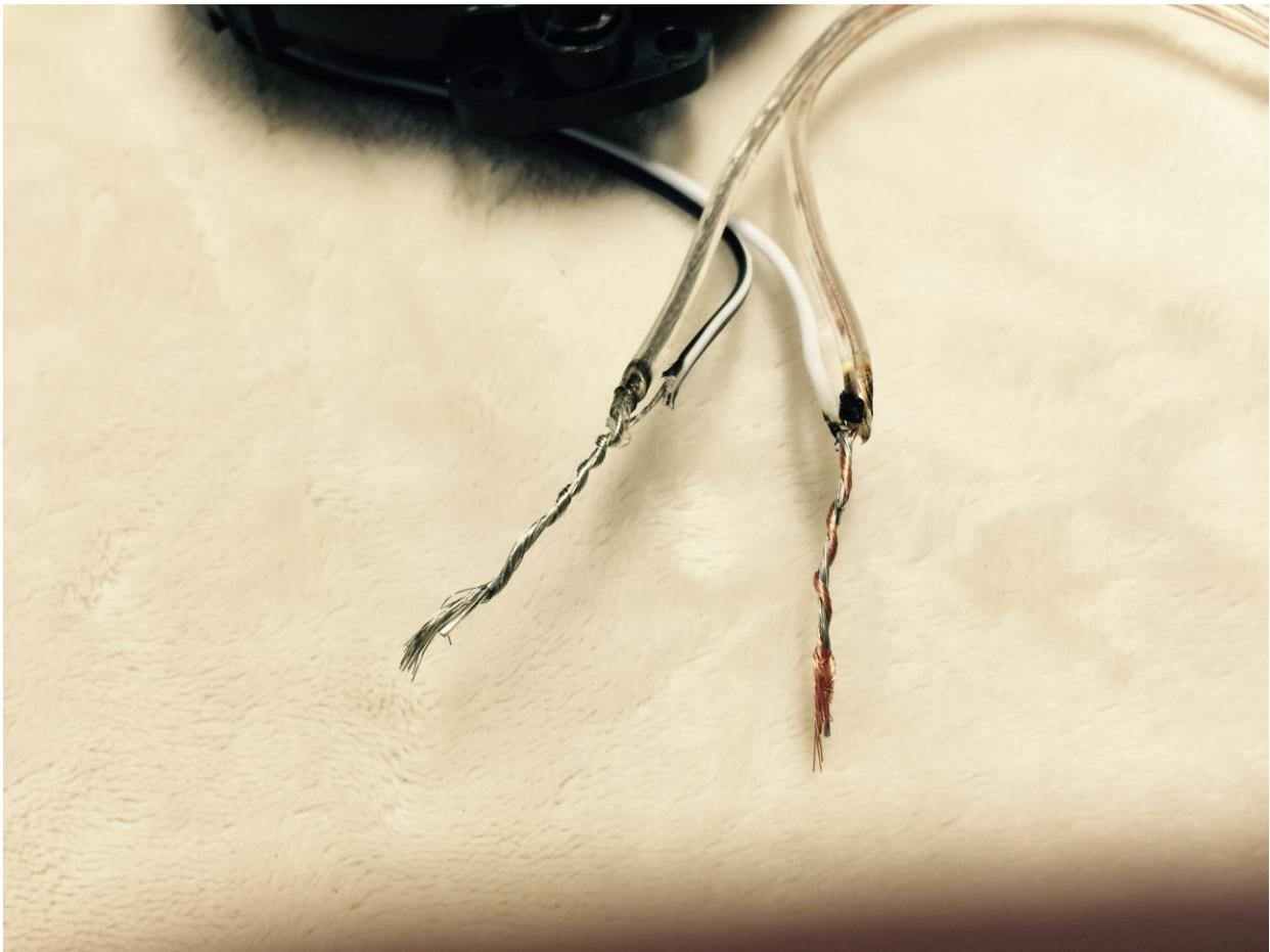
Now that the one inch exposed wires are twisted together, fold the twist in half to make them 1/2 inch wires on all ends of the additional strands of speaker wire. Twist the two halves together to for one short 1/2 inch wire. We will discuss the ends that go into the amplifier later.
