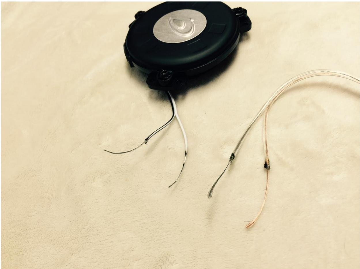
**Important:** Now join the ends of the striped wires by twisting them together. **Twist the white wire (positive +) on the puck to the gold/copper colored wire (positive +) on the speaker wire you cut** then **twist the black wire (negative -) on the puck to the silver wire (negative -) on the speaker wire you cut.**
