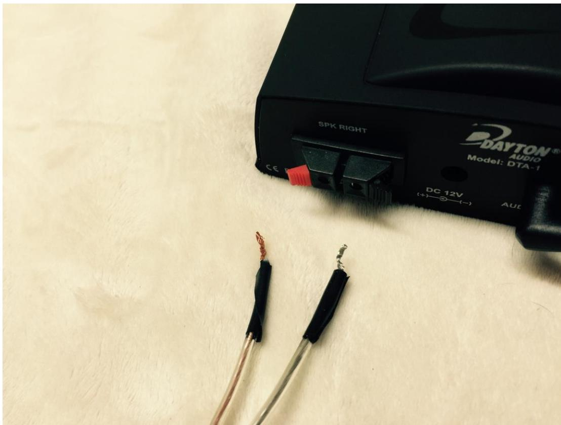
The receptors for the speaker wires on the back of the amplifier are red and black; **red is positive and black is negative.**
